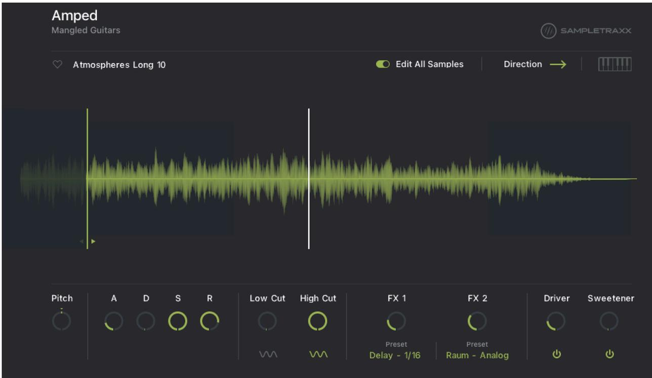
In the image above, the Sample Start has been adjusted to a later start position in the waveform view. You will want to increase attack time to prevent an unwanted pop at the start of playback. *Note: When in Global Mode, this will affect all samples within the instrument.*
