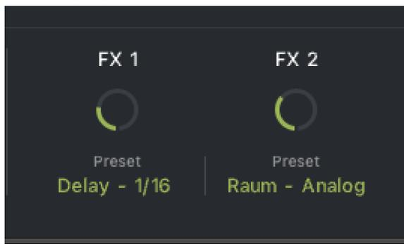
There are two dynamic effects modules - **FX1** and **FX2** - that load and control instrument effects. These effects can be applied to all samples at the same time or individually when not in global mode. Choose from Chorus, Delay, Flanger, Phaser, Plate (reverb), Psyche Delay, Raum (reverb), Replica (delay), Twin (delay). Use the dropdown menu to load/switch effects.
